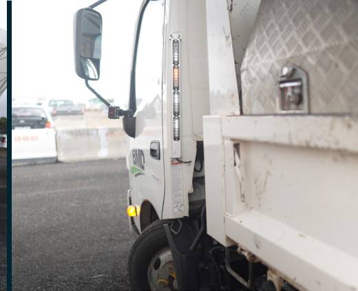
The AI smart camera is installed on the left side mirror and position to view the driver blind spot areas (left), when activated an audible message is sounded and the light bar flashes (right).
